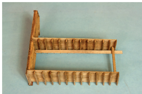
7. One side of the beam is in place. Rather than doing things the hard way and installing all of the posts first, installing one side of the header first will serve to align the remaining posts. The overhang at the end was left to possibly tie the shed into the main building. If this does not work out it can always be trimmed later.
